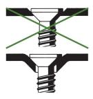
Plugs for mounting bolt have special interlock, which makes place of connection more durable.
