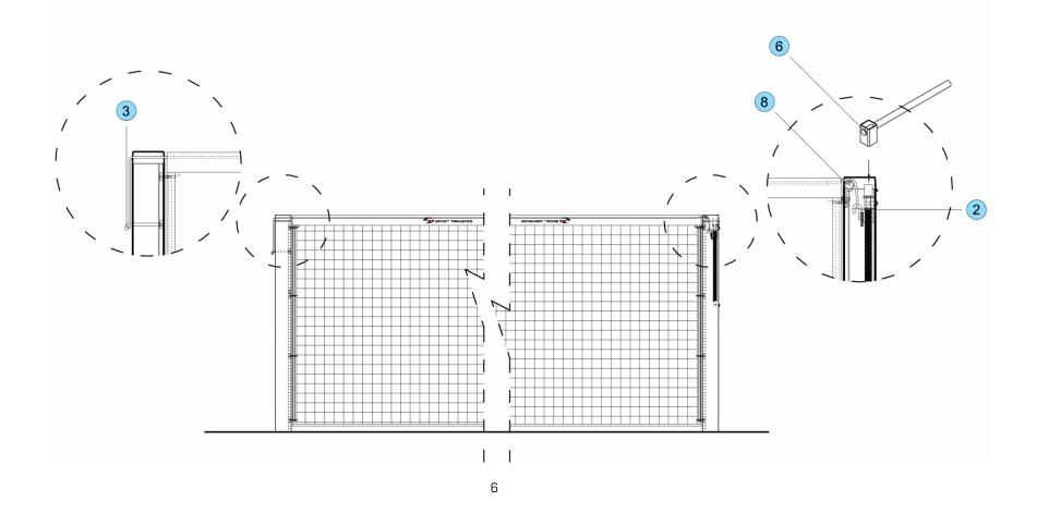
d) After tensioning the suspension line, tension the net with the tension rods (5) put through the meshes of the net and the hooks of the rods (4) and tie the tension cords to the top of the posts so that the net is symmetrically aligned towards the transverse axis of the court.
