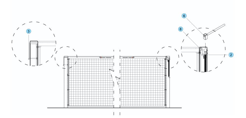
d) After tensioning the suspension line, tension the net with the tension rods (5) put through the meshes of the net and the hooks of the rods (4) and tie the tension cords to the top of the posts so that the net is symmetrically aligned towards the longitudinal axis of the court.
