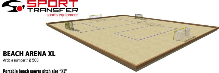
Special system of sideboards folded on any flat surface to form a closed body covered with sand. 40cm high sideboards of the pitch made of 10mm thick polyethylene panels fixed to special steel supports. Hot-dip galvanised and powder-coated
