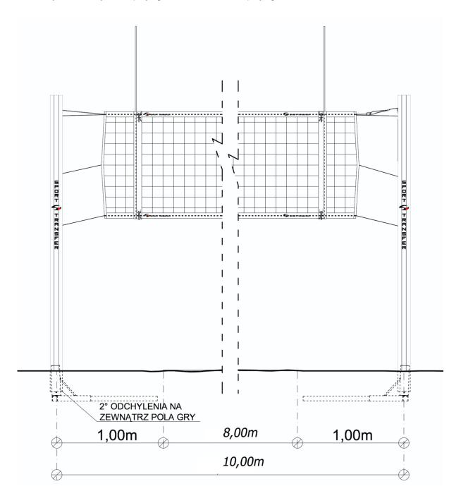
b) The upper edge of the sleeve should be about 50mm above the sand level. Before filling the sleeves (6), it is recommended to weight additionally the beams (7) with sandbags.
