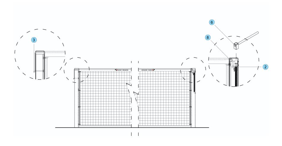
d) After tensioning the suspension line, tension the net with the tension rods (5) put through the meshes of the net and the hooks of the rods (4) and tie the tension cords to the top of the posts so that the net is symmetrically aligned towards the longitudinal axis of the court.
